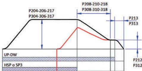
In this case, at the slowdown contact, is performed a deceleration space equal to the parameter set for normal stroke which however considers the speed reached in that moment, operating if provided (P456 = 1), also the corrections of the usual slowdown and low speed spaces.
