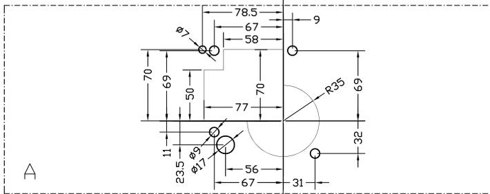
Plate mounting hole/shape pattern
