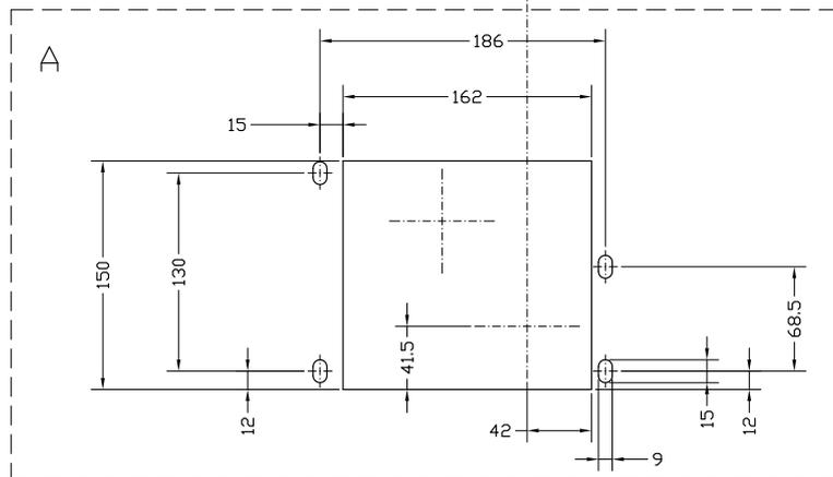
Plate mounting hole/shape pattern
