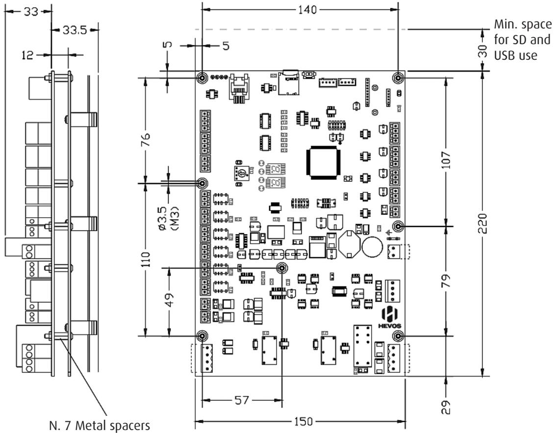
Board fixing metal plate 1.5 mm for DIN 35 bracket
