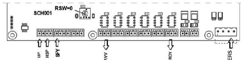
Once finished the motor starting (direct, star-delta or soft starter) the control panel must return a signal to SFY board input. If the SFY signal is not available, it is useful to adjust the parameter P403 which sets the valve pre-starting time, after which, however, the valve unit executes the starting phase.
