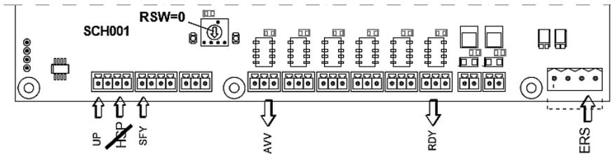
Upon arrival to the deceleration contact in the elevator shaft, turn off the high speed HSP signal and the valve unit executes the deceleration curve set up in the parameters P207, P208 (209,210,218) and P211 to obtain the low speed value corresponding to P212 parameter.
