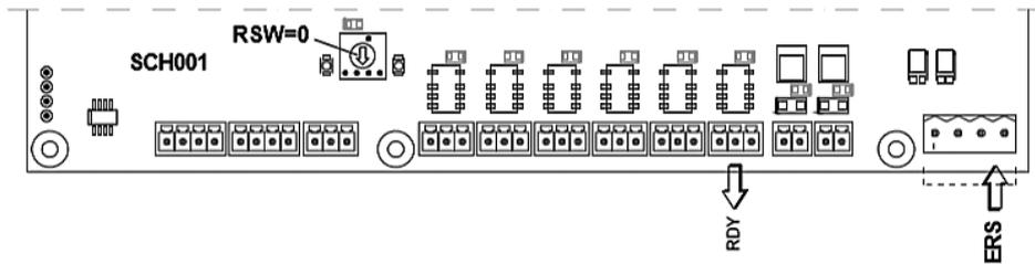
Power input of only solenoid valve ERS.
