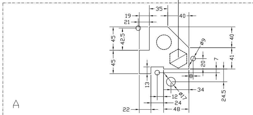
Plate mounting hole/shape pattern
