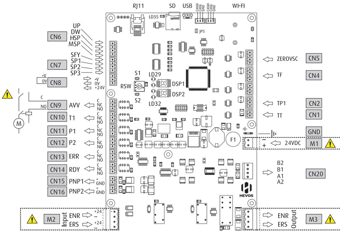
**ATTENTION:** Reversing the polarity on the **24VDC stabilized power supply**, or inversion of M2 and M3 connectors, will irreparably damage the board!
