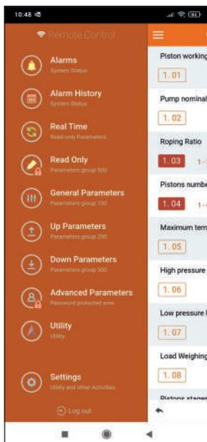
**Alarms:** errors/reports of the active installation at the reading time.
