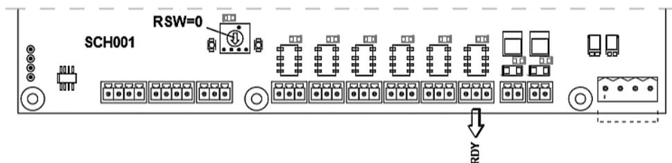
Ready signal RDY from the board to the electrical panel waiting for commands or ERS valve activation. The board goes in error (error code = 19, DSP = E3) if the waiting time signals exceeds 12s.
