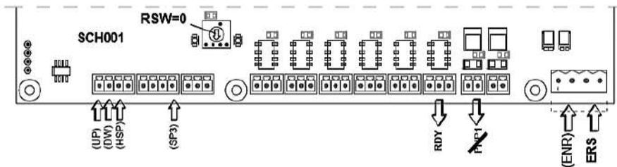
The signals in parentheses are used together or alternatively as in normal manoeuvres.
