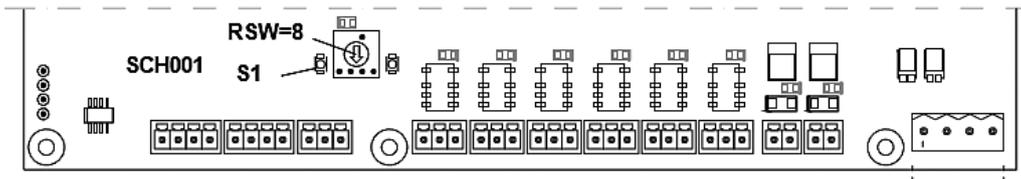
Block the system to exclude the possibility of travel. Set the working selector RSW = 8 (DSP= PP) and then press S1 button until appear HP on display. This prepares the valve unit to execute the next upward working cycle with a progressive pressure starting and without flow error condition. Close the ball valve.
