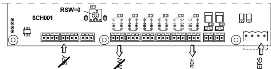
If during the starting phase it has not been used the AVV motor contact activation, delay the stop of the motor of 1.5 s, otherwise when the signal AVV turns off, stop the motor (and then the input signal SFY). Anyway, do not delay the stopping of the motor more than 2 s from the arrival to the stopping contact in the shaft.
