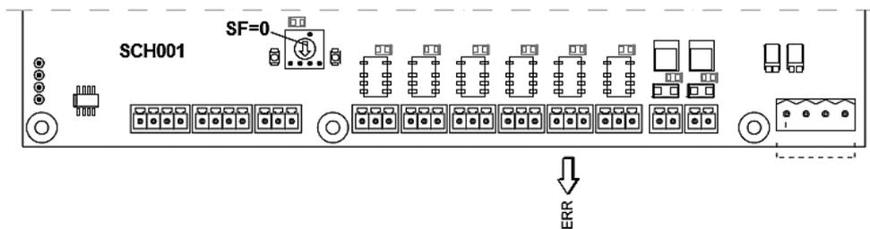
Any operation shall be prevented if the error signal on the ERR relay is active. For error handling see the section “Parameters and errors codes”. You can force on the error condition the signal ERR by disconnected the CN5 connector. This allows to verify the block of the control panel to the switching-on of the error signal ERR.
