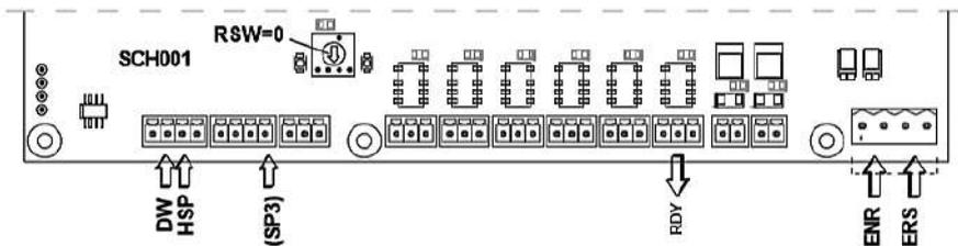
Activation of Downward DW and high speed HSP (or SP3 if the parameter P453=1) command input and power supply of the solenoid valves ENR and ERS. The HSP (or SP3) high speed command can be replaced by MSP maintenance command (P454=0) or work together to signals MSP (P454=1), SP1 or SP2 to determine different values of high-speed set in the corresponding parameters.
