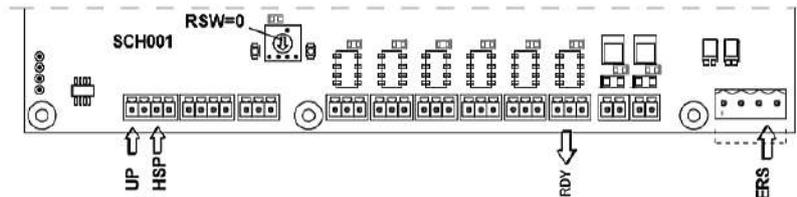
Activation of Upward UP and high speed HSP command input and power supply the solenoid valve ERS. The HSP high speed command can be replaced by MSP maintenance command (P454=0) or work together to signals MSP (P454=1), SP1 o SP2 to determine different values of high-speed set in the corresponding parameters.
