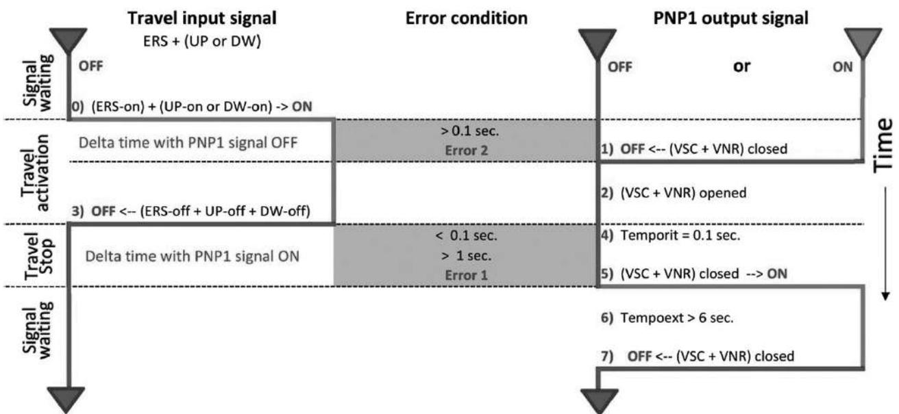
1. At the start of the manoeuvre, when the INPUT (ERS+UP) or (ERS+DOWN) are activated if within 0.1s there is no PNP1=OFF to indicate that the VSC and VNR valves are closed, it generates Error2 (E2).
