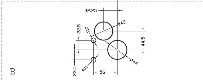
Pump tube mounting hole pattern
