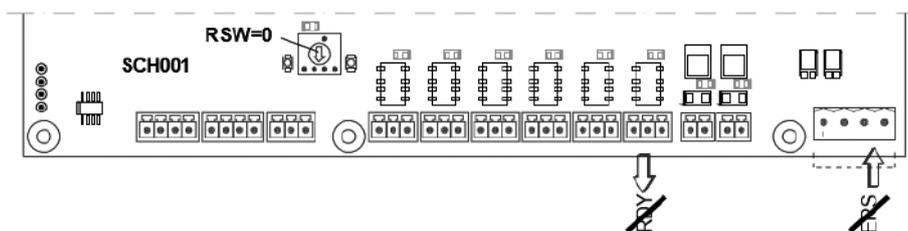
Subsequently the shutdown of the RDY board signal also remove the ERS solenoid input. The RDY board signal is active again after about 0.5 s, when the valve unit will be ready for the next travel. However, remove the ERS solenoid input after 2 s from the arrival to the stopping contact in the shaft
