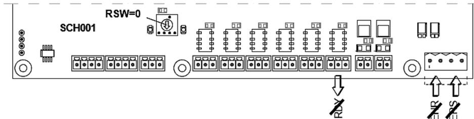
Subsequently the shutdown of the RDY board signal also remove the ERN and ERS solenoid inputs. The RDY board signal is active again after about 0.5 s, when the valve unit will be ready for the next travel. However, remove the ENR and ERS solenoid inputs after 2 s from the arrival to the stopping contact in the shaft.
