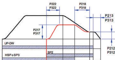
In this case, the HEVOS system uses the SP2 input and the HSP input (high speed) together with the direction control (UP, DW) operating, if provided (P456=1) also the corrections of the slowdown and low speed spaces.
