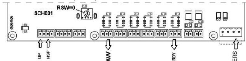
The board commutes the AVV output to give consent for motor pump starting. In this phase, the pump oil flow is discharged in the tank at low pressure to allow a proper motor starting and avoid hit in the cabin caused by pump direct flow to piston.
