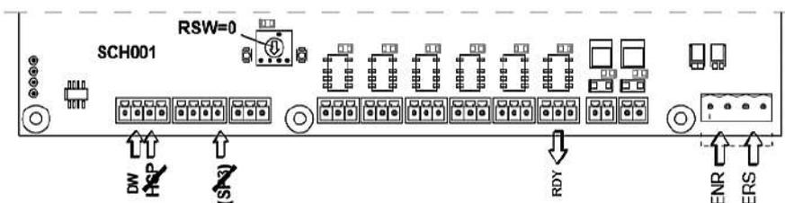
Upon arrival to the deceleration contact in the shaft, turn off the high speed HSP signal (or the SP3 signal if the parameter P453=1) and the valve unit executes the deceleration curve set up in the parameters P307, P308 (309,310,318) and P311 to obtain the low speed value corresponding to P312 parameter.
